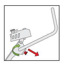
THE MACHINE IS EQUIPPED WITH TWO LOCKING MECHANISMS — ONE FOR THE HANDLES AND ONE FOR THE WHOLE HANDLEBAR.
