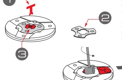
USE THE TOOL HOLDER KEY /1 / TO ROTATE THE KEY LOCK /3 / In order to unlock and remove security plate /2/.
