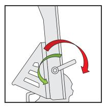
TOROTATE THE WHOLE HANDLEBARUSE THE LEVER (RED ARROW FOR LOCK DIRECTION) AND (GREEN ARROW FOR UNLOCK DIRECTION).
