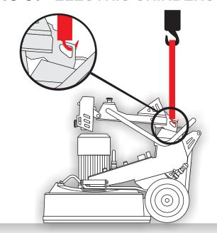
TO TRANSPORT THE MACHINE, USE THE HANDLES OF THE GRINDING HEAD AND THE REAR BAR AS ANCHORING POINTS FOR STRAPPING THE MACHINE DURING TRANSPORTATION.
