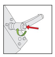
THE HANDLE IS ADJUSTABLE. TO SET IT INTO MORE CONVENIENT POSITION PRESS THE BUTTON AND ROTATE THE LEVER.
