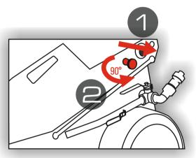
TO MOVE THE WEIGHTS, RELEASE THE LOCKING KNOB BY PULLING IT, AND THEN RELEASE IT TO LOCK INTO THE NEW DESIRED POSITION.
