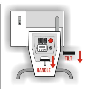
THE MACHINE IS EQUIPPED WITH TWO LOCKING MECHANISMS — ONE FOR TILT AND ONE FOR HANDLE ADJUSTMENT. PULL THE LEVER TOWARDS OPERATOR TO UNLOCK AND ADJUST TILT / HANDLE TO DESIRED POSITION. THE MECHANISM LOCKS ITSELF BACK.
