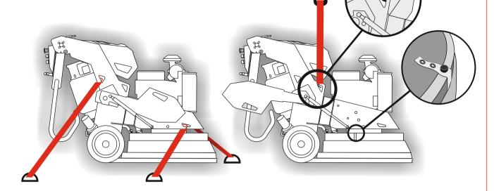
LAVINA MACHINES HAVE FOUR ANCHORING POINTS FOR STRAPPING DURING TRANSPORTATION. MAKE SURE MACHINE IS SECURELY ANCHORED, AND GRINDING HEAD COVER IS LOWERED DOWN / LOCKED. TIGHTEN THE STRAPS OVER NON-MOVING PARTS, E.G. MACHINE CHASSIS.
